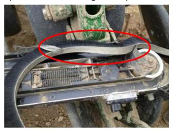
Separation greater than 2.5cm (1 inch) may still operate but should be replaced if performance is affected
